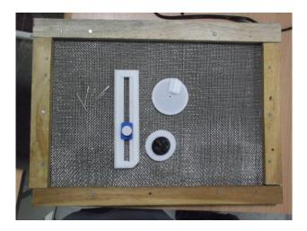
We also built a mesh based tactile board with multiple mesh layers to help us test the instruments. We had decided to use dressmaker's pins to set a frame of reference for the blind students who would use it.
